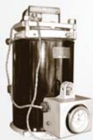
Dr. Kesling made his first tooth positioners with this S. S. White Steam Vulcanizer.
